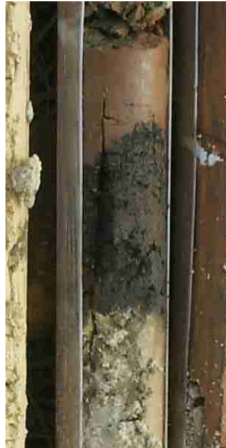
Fig. 3 DARAMEND layer injected between clay and weathered limestone.
