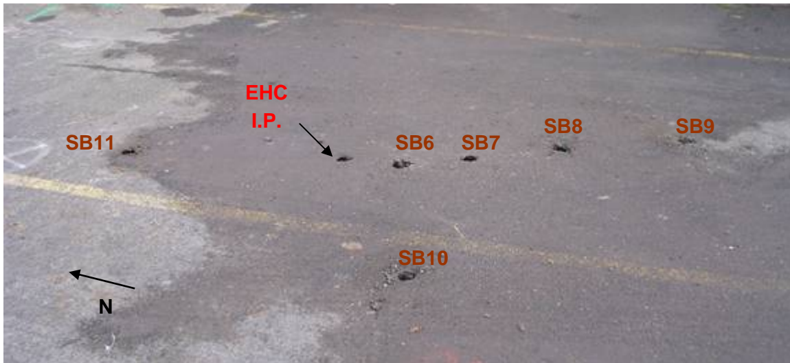
Figure 1: Soil sampling locations around EHC injection point.
