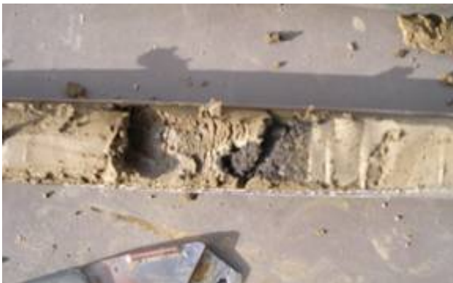
Figure 2: EHC fracture at 17.5 ft bgs (SB6).
