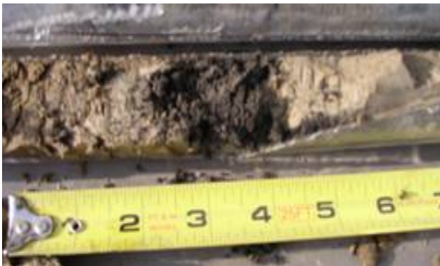
Figure 4: EHC fracture at 17 ft bgs (SB7).
