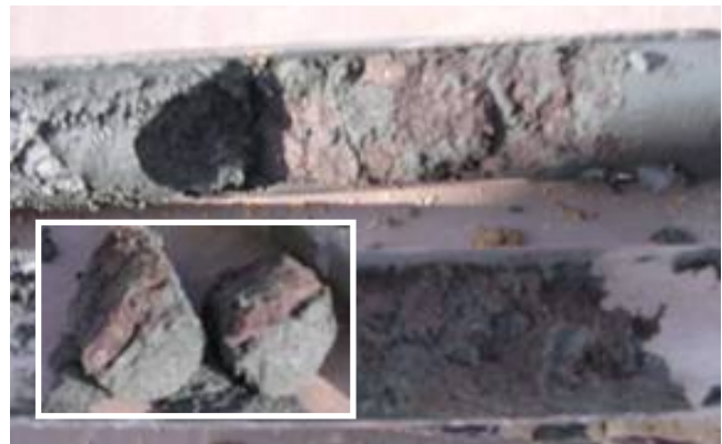
Figure 3: Vertical EHC fracture at 26.8 ft bgs (SB6).
