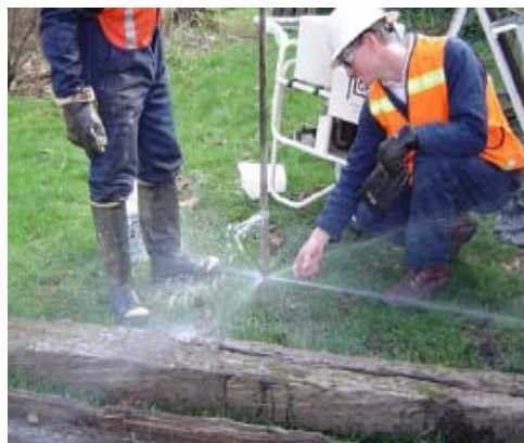
Test of pressure activated tip with 4 horizontal openings.
