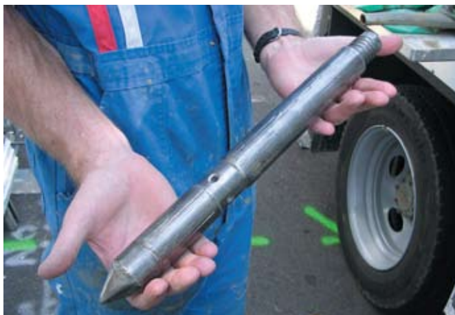
Exhibit 1. Pressure-activated injection tip with four side injection ports.
