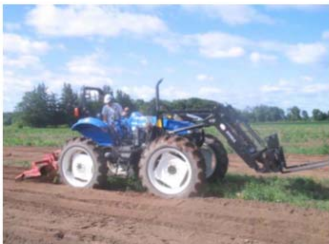
Figure 4: Incorporation of DARAMEND into soil using specialized tillers.
