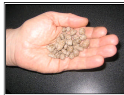
Figure 4. AquaBlok HoleBlok™ and HoleBlok+™ grout particles are easy to handle and place. No mixing or special equipment is required.
